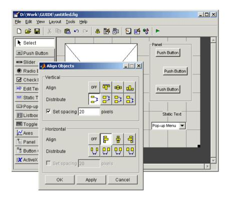
Now align the tops of the axes and the panel. Note that when the panel moves, its contents move with it.
