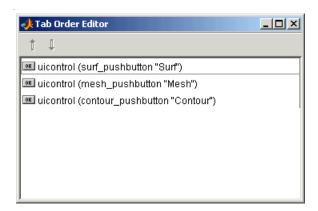
The Tab Order Editor displays the panel's components in their current tab order. To change the tab order, select a component and press the **up** or **down**
