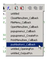
Clicking a callback on the list displays the section of the M-file containing the callback, where you can edit it. This example shows the callback template for pushbutton1\_Callback.
