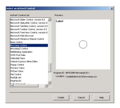
**3** Click **Create** to display the ActiveX control in the Layout Editor, and resize the control to approximately the size of the square shown in the preview pane. You can do this by clicking and dragging a corner of the control, as shown in the following figure.
