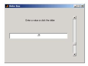
Defining the Data Fields in the Opening Function. The GUI records the number of times a user enters an erroneous value in the text box and stores this number in a field of the handles structure. Start by defining this field, called number errors, in the opening function as follows:
